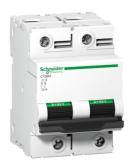
Acti9, Miniature circuit breaker (MCB), Acti9 C120H, 2P, 100A, C curve, 15000A (IEC/EN 60898-1), 15kA (IEC/EN 60947-2)
